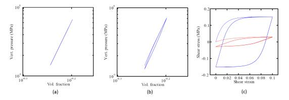
**Figure 1:** (a) Biaxial transverse compression, 10% volumetric, two cycles starting at  $\phi_0 = 0.57$ , (b) Uniaxial compression, 10% volumetric, two cycles starting at  $\phi_0 = 0.57$ , (c) Two cycles of 10% longitudinal and transverse shear strain.
